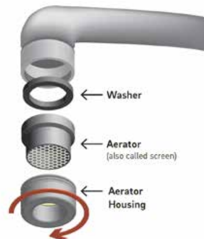
FIGURE 5 Diagram of faucet aerator
