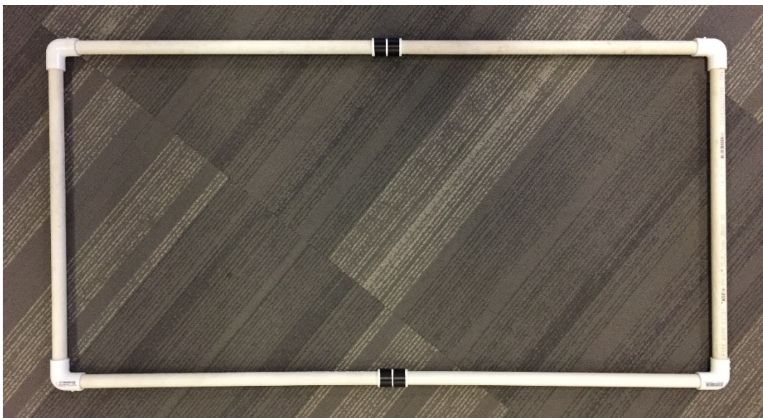
Figure 16. Subplot frame used to collect field data for the Monarch HQT. The subplot frame is a 0.5 x 1.0-meter frame, divided into 2 subplots; the final (3 rd ) subplot results from flipping the subplot frame over
