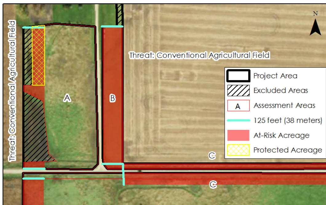
Figure 9. In Assessment Area A, a double-row hedgerow (which was excluded in Step 1), is protecting much of the habitat from pesticide drift. The area protected by the hedgerow was delineated (indicated in the yellow cross hatched area) and the area in acres calculated.
